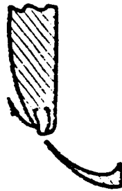
BLOWING- SLOTTED FLAP
